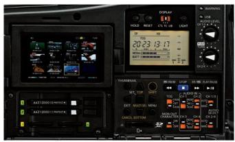
Card slot, LCD monitor and recorder-related function parts
