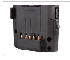
S-7010S adopts new robust thickened power pins, fully contact with batteries, and reduce the contact resistance from  $2.4 \text{m}\Omega$  to  $0.8 \text{m}\Omega$ , to ensure safety when high current pass through from battery.
